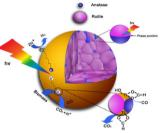
For photocatalytic biomass reforming on Pt/TiO<sub>2</sub> by tuning anatase-rutile phase structure, the hydrogen production activity can be significantly enhanced and CO concentration can be reduced from thousands ppm to 5 ppm.
