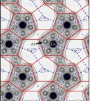
Electron density distribution in the catalytically active (100) surface of Al<sub>13</sub>Co<sub>4</sub>.
