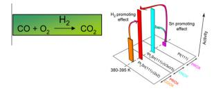
Both Sn and  $H_2$  promote CO oxidation on  $Pt_3Sn(1\ 1\ 1)$  surfaces. The surface structure sensitivity in CO oxidation is cancelled out when the reaction is performed under a large excess of hydrogen.
